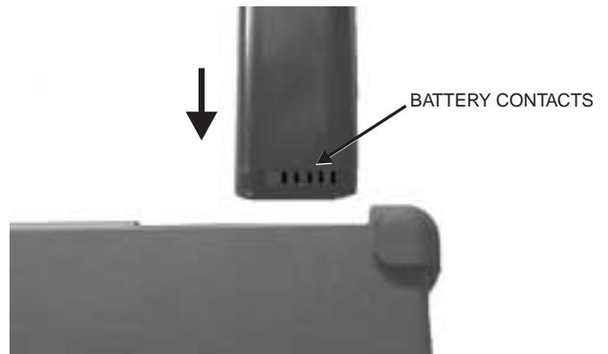
**Figure 10.** Battery Orientation
