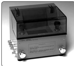
Agilent 42842A/B/C bias current test fixture
