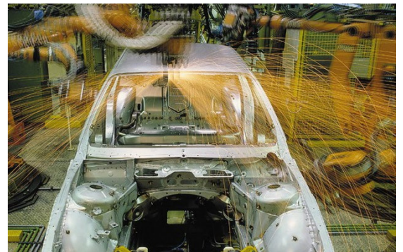
Resistance welding machinery in operation
