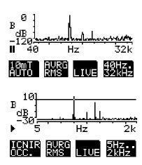
The EFA-300 is so powerful that even transient events ranging up to 2 kHz can be analyzed in real time.
