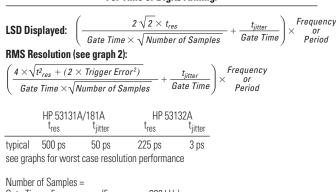
Gate Time x Frequency (Frequency < 200 kHz) Gate Time x 200,000 (Frequency > 200 kHz)
