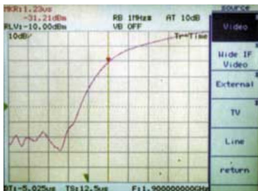
High-speed time-domain measurement (TS=12.5 \mu s)
